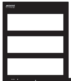
2. Place the 12" x 3 1/3" industrial film to be scanned inside the frame of the film holder, with the correct side facing up.
